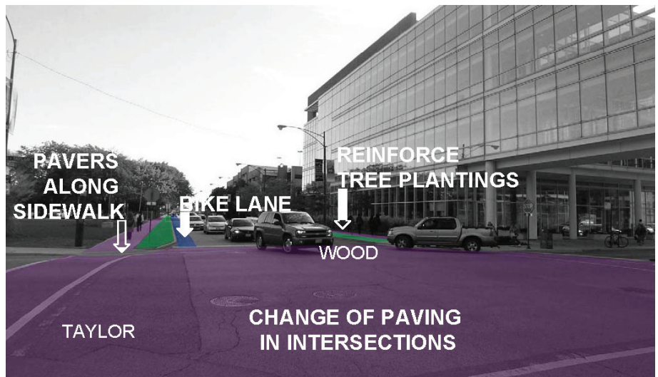
Campus Street - Narrowing Wood Street will discourage high speed vehicular travel and encourage pedestrian use.
