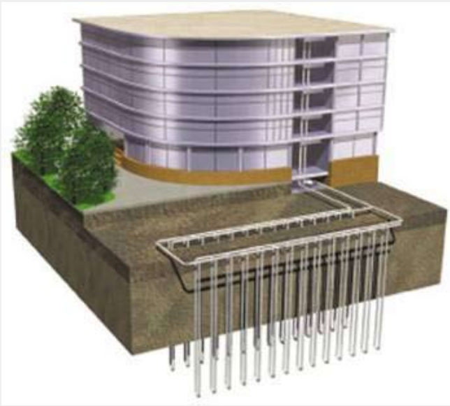
Figure 81.1 Geothermal heating and cooling
