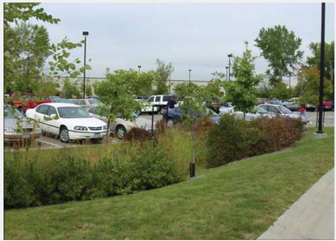
Figure 81.4 Bioretention swales/stormwater run-off management
